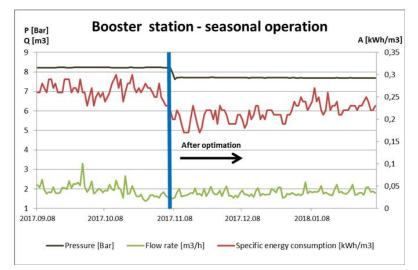
Figure 5. Optimized pumping station with lower winter pressure
