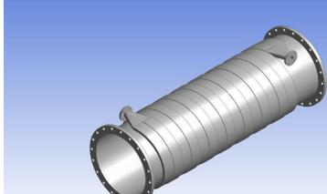
The new heat pump's main innovation is its concept by using the drinking water pipe as heat exchanger. Furthermore, its parameters were exclusively set to the pressure side of the pumping station. The pipe is covered by a casing where circulation of the secondary fluid doesn't create any additional pressure lost while the free heat capacity of the drinking water is exploited. The helical external casing can maximize the residence time without stagnant areas.
