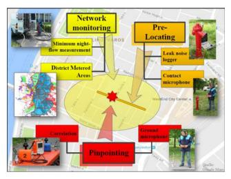
Figure 1. Leak detection methods and instruments
