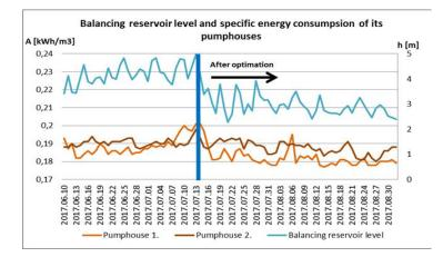
Adapting the operation of pressure zones to consumer habits (e.g. setting day/night pressure): At all periods the lowest pressure level has to be defined which is still sufficient to supply the given zone. Pressure reduction may also cut back NRW, which is an additional advantage.
