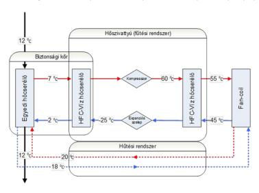
The image here below presents the layout of the unique heat pump system designed by Budapest Waterworks professionals.
