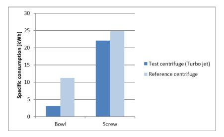
Figure 2. Comparison of the specific energy consumption of the existing and the upgraded centrifuges
