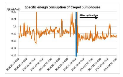
Figure 3. Specific energy consumption of Csepel pumphouse
